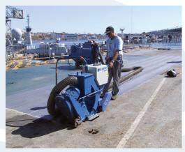
Production rates achieved will be affected by variables specific to each job site. These figures are not guarantees of performance. For proper operation, the shot blasting unit must be used in conjunction with an appropriate dust collection device.
